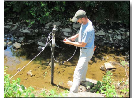
Checking data logger installations
